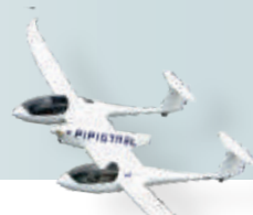
Taurus G4 world's first four seat electric aircraft
