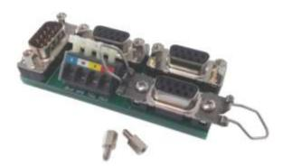
After that small modification, fixing the Trig Bridge to the RS485 splitter will be very easy.
